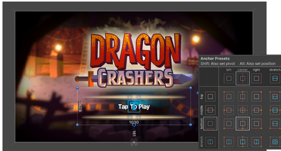
The selected Rect Transform is anchored to the bottom/center of its parent Rect Transform, with a gap of 161 pixels from the bottom and 0 pixels from the horizontal center.
